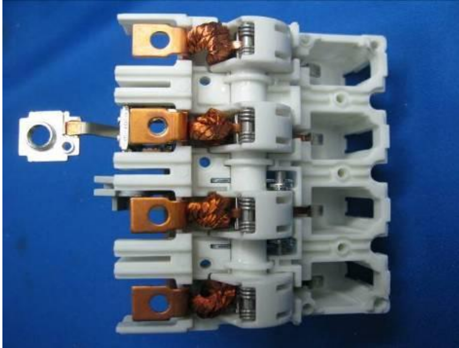
Box of contact, 3P + N, MCCB
