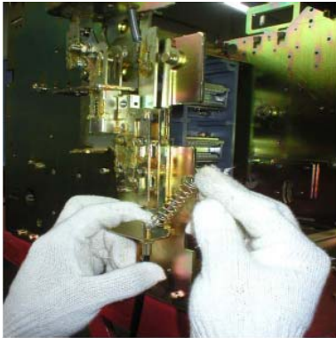
20-8. ASSEMBLE N-ME-CABLE-BUSH2 IN THE DIRECTION OF DEEP HOLLOW
